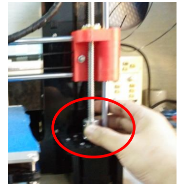
Fig 4: measure height of X-slide
