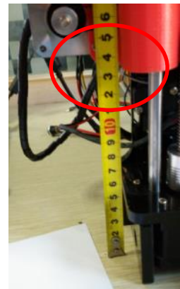
Fig 4: measure height of X-slide
